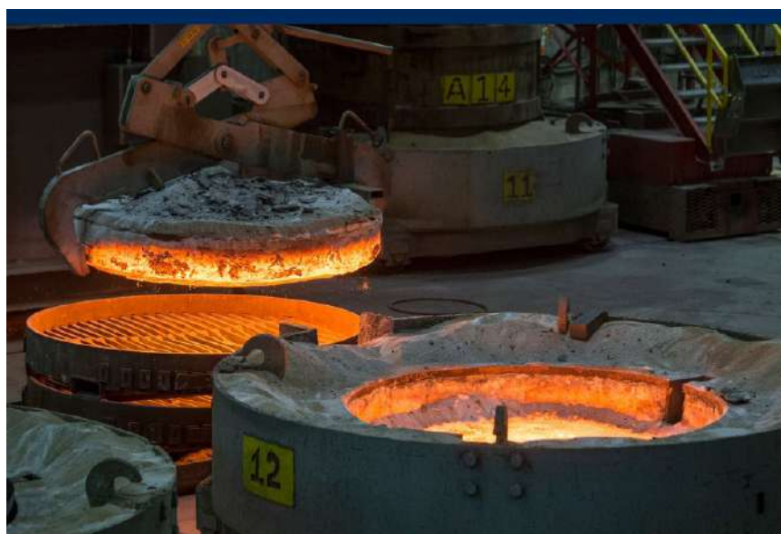
Figure 10 Ferroniobium billet being removed from a converter at Niobec
