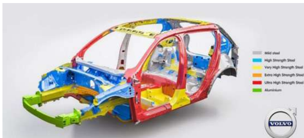
Figure 6 Automobiles use High Strength Low Alloy (HSLA) steel in the vehicle body
