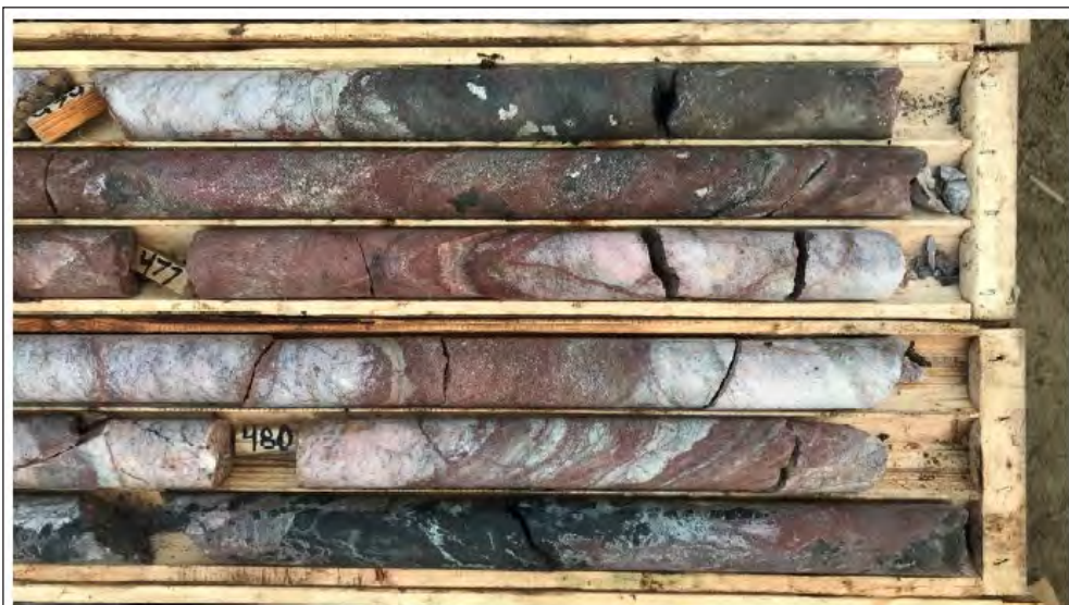
Figure 3: Diamond drill core (NQ, approximately 4.8 cm diameter) from hole POM-23-09 containing abundant visible REE mineralisation (dark red colour) hosted within calcio- (pale) and silico-carbonatite (dark). Approximately 474 to 482m down hole.
