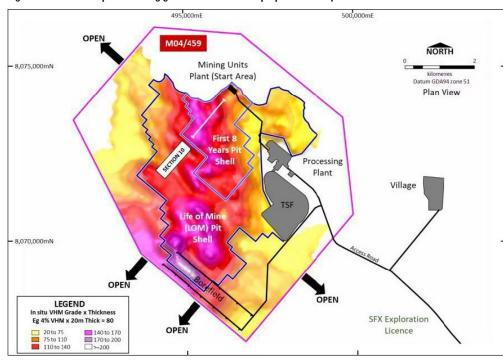
Figure 6: Thunderbird plan showing grade x thickness and proposed site layout
