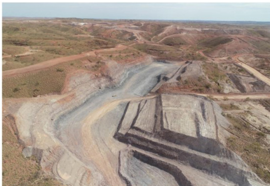
Figure 16 Grants Hill in the foreground with the fresh mineralisation dipping to the left and the oxide pits in the background
