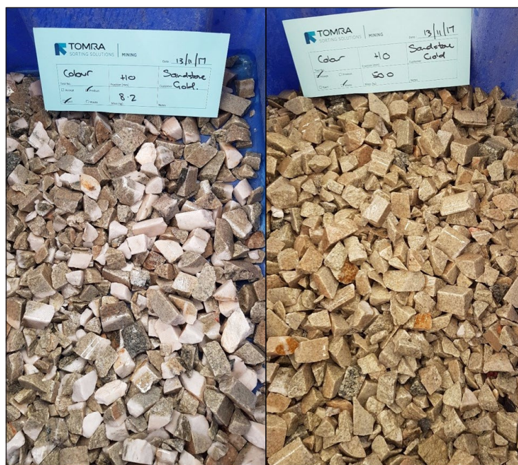
Figure 4: Initial Two Mile Hill ore sorting - vein material (L) and rejects (R)
